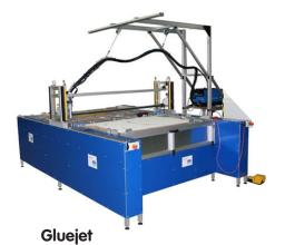
Utilising versatile and accurate gluing systems is vital to producing top-class POP and the latest Bickers Gluejet (X and Y) adhesive table, which is a 2000mm x 3000mm configuration, now meets the ever-growing needs of this fast-expanding business. It's an automatic plotter that applies hot melt and PVA glue within the same programme on up to four separate work stations.
